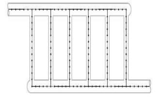
Figure . Pseudo-1D mesh of a simple flow system
