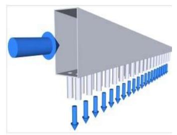
Figure. Distributor with variable rectangular cross-section and double lateral branches
